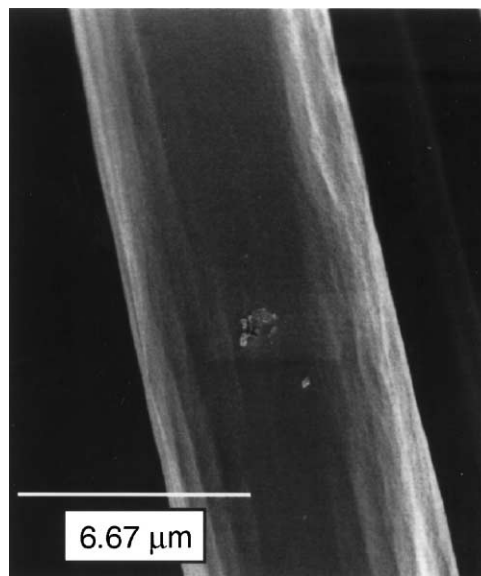
Fig. 4. Fibre surface of a carbon fibre in a N preform which has been successively treated with H_3BO_3 , washed with distilled water and finally oxidized.
